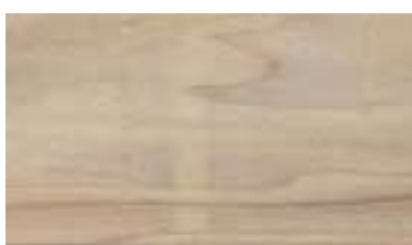
STICKER MARK: The mark left on the board from a seasoning sticker, which can be removed in the surfacing planing process.
