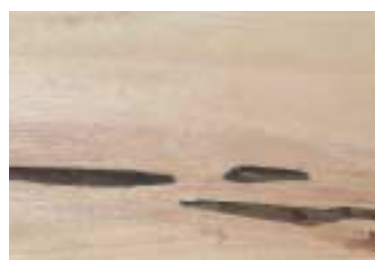
GRUB HOLES: Holes larger than \frac{1}{4} "
