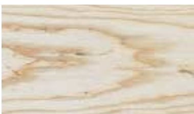
GLASSWORM: Random mineral like tracts. Usually associated with ash
