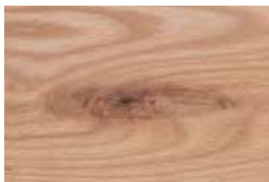
BARK POCKET: A bark-filled distortion in the grain pattern.
